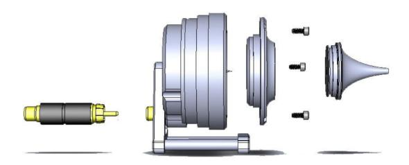
MF1 Closed Field Speaker Assembly Diagram
