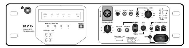
The RZ6 Multi I/O Processor provides the processing power for averaging signal inputs and the digital-to-analog converters and amplifiers for producing the stimuli. It also provides the precise timing essential to evoked response experiments. The power input and optical connection to the PC are located on the back. The input/output support (such as speaker drivers) and attenuation that is incorporated into the device are all accessed on the front panel.
