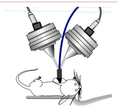
To minimize the effects of distortion or interference, keep ear tubes short to minimize bending and prevent crimping. TDT recommends positioning the subject on it's side and mounting stimulus speakers directly above the subject's ear- allowing for tube lengths of 3 - 5 cm and repositioning or turning speakers as needed rather than bending ear tubes.
